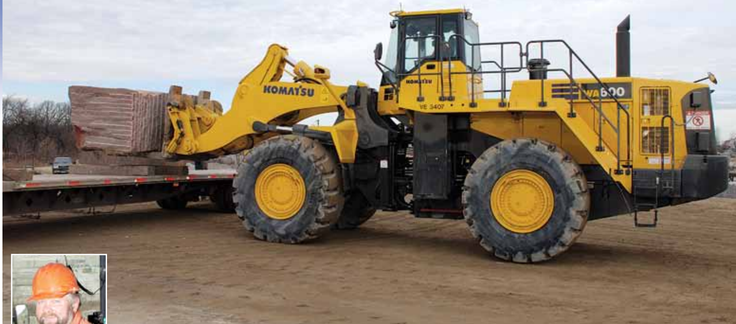
Operator Ervin Klehr loads a granite block onto a trailer with one of Cold Spring Granite's newest Komatsu WA600-6 wheel loaders at the Rockville No. 2 Quarry. "Because we deal with large rectangular blocks of granite, we need machines that can lift at least 80,000 pounds," said Jim Fuchs, Engineering and Quarry Equipment.
