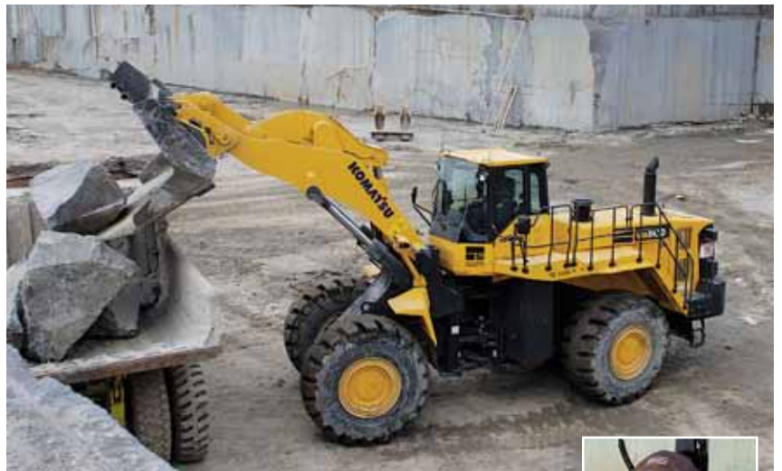
Operator Dean Forster uses a Komatsu WA600-6 wheel loader to put stone in a truck at Cold Spring Granite's Charcoal Quarry in St. Cloud.
