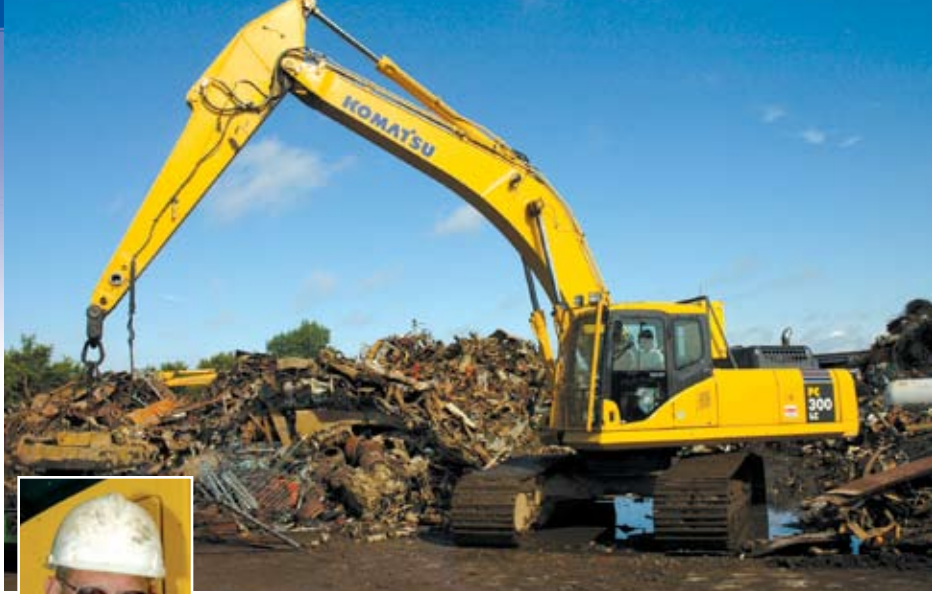
Operator Paul uses a Komatsu PC300LC-7 equipped with a magnet to unload scrap metal from a customer's trailer. "I like the way it handles," Paul said of the PC300. "It has good hydraulics and will pick up a lot of weight."
