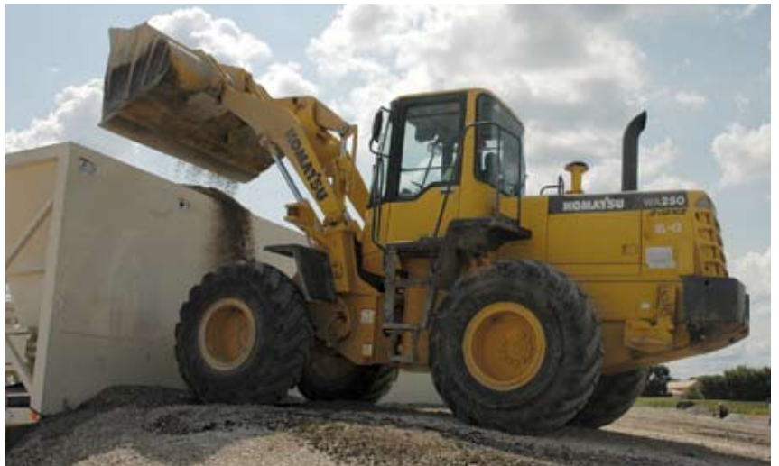
Eco-Tech relies on Komatsu wheel loaders in its paving operations, including this WA250 used to load a hopper at the company's new asphalt plant in Grimes.
